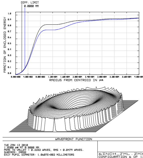
**Figure 4. The fraction of encircled energy (top) is shown with respect to the diffraction limit. The wavefront error map is also shown (bottom) to convey the nature of the residual design error. These are shown for the optics set to focus at a distance of 3km, where the beam size is approximately 1.2 meters in diameter (due to the extended size of the fiber source, this is larger than a point source).**
