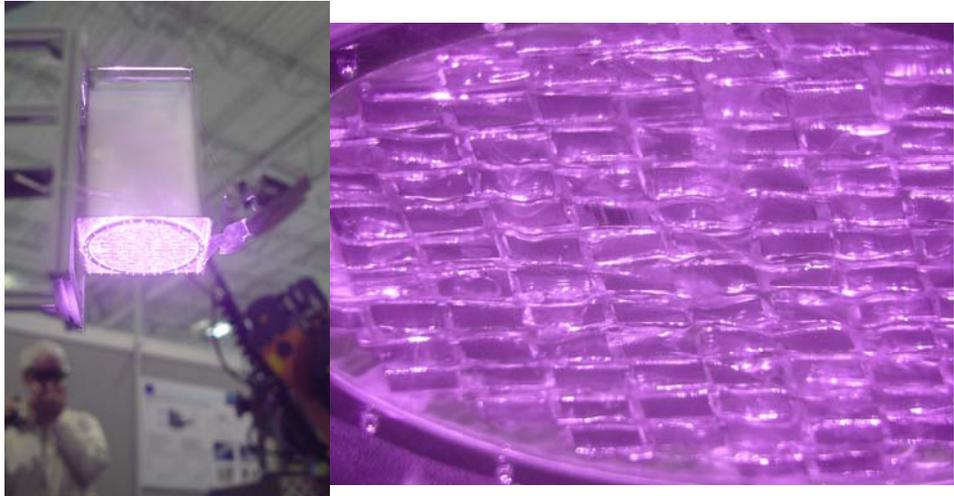
**Figure 7. The TPV array being “melt” tested at Trumpf Laser, illuminated from below. A close-up view (right) shows the bubbling acetone maintaining the cells at a constant temperature of 56°C.**
