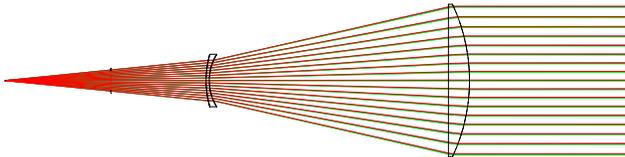
**Figure 3. This shows the layout of the Beam Forming optical design. Both lenses are catalog off-the-shelf available through JML Optical, and produce a nearly diffraction-limited beam at 1032nm. Although rays are shown here to the edge of the lenses, approximately 95% of the laser energy resides within the central 112mm of the outgoing beam.**
