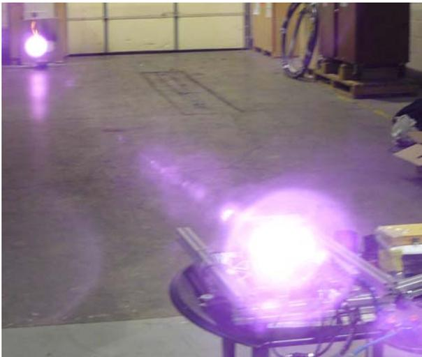
**Figure 8. A picture at a time of approximately 10 seconds after the transmitter optics “melt” test commenced. The beam dump is a series of gypsum boards, the paper of which ignites (seen here) and burns away, leaving the bare gypsum for the beam to dump into.**
