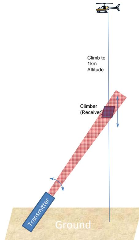
**Figure 2. Depiction of the power-beaming Centennial Challenge. The transmitter sends power via laser beam to the vehicle climbing the tether.**
