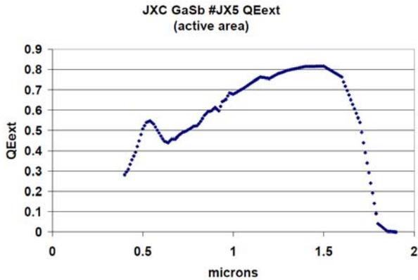
**Figure 6. Quantum Efficiency curve for the TPV cells. Data provided by the manufacturer.**
