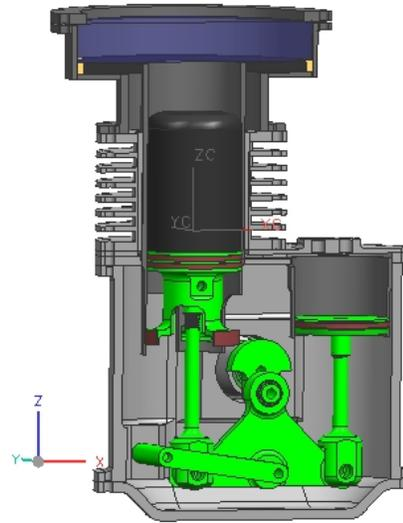
**Figure 5. A cross-sectional view of the Stirling engine design that was developed for this challenge, however schedule complications led to the design being abandoned. It is currently being reconsidered for a future competition.**
