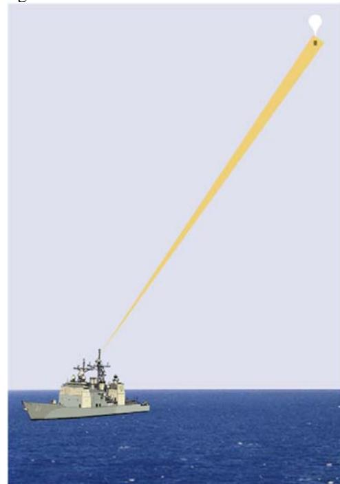
**Figure 1. A possible use-case of power-beaming: sending power to a payload on board a high-altitude balloon gondola.**
